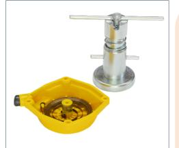
The wrapped rewind spring is ready for use inside the starter cover.
