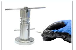
After the cup-washer set is installed, remove the lock pin. Ready for use.
