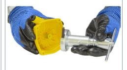
As soon as you tighten the upper and lower shafts, the rewind spring will be released from the cup. To do this, first put the spring into the cover or rewind spring cup where you will place it.
