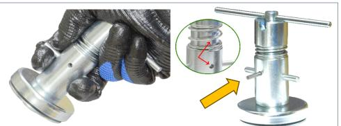
Replacing the Cup and Washer: Squeeze the winder in your hand between the upper and lower shafts. Align the outer casing and inner casing fixing holes according to the guide line and insert the lock pin.
