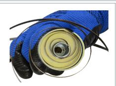
Insert the inner end of the discharged spring through the slot in the center of the winder. Make sure that the other remaining end is on the table outside the outer slot.
