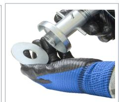
First remove the washer on the winder. It is the right pass.
