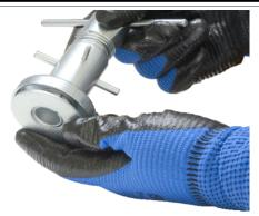
Pass-fit first the cup and then the washer of the cup-washer set of the size you want to use
