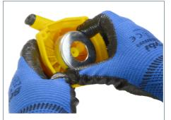
Find the appropriate cup-washer set according to the size of the place where the rewind spring is to be installed.
