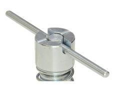
**Usage of Winder:** The upper winding shaft should be in the deep groove. The spring to be wound can be wound on a suitable table.
