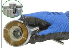
When the winding is finished, pull the upper winding shaft out of the deep groove and insert it into the upper small groove. This will free the core of the spring from the groove.
