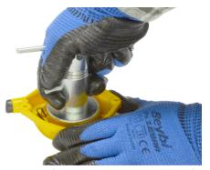
Then carefully squeeze the winder shafts in your hand and place them where the rewind spring will come out of the winder and work.
