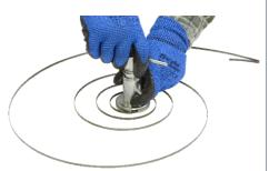
Secure the rewind spring winder on the table with one hand. Wind the spring into the cup by turning the upper shaft to the right or left, depending on where the spring will be used.
